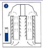
With increasing dust deposit, the filter resistance increases. As the set-up differential pressure is reached, the cleaning cycle begins automatically.
