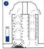
Undisturbed continuous operation is ensured by the single cleaning of filter elements. The dust falls back into the silo. At a under usage of a minimum-filter resistance, the cleaning cycle turns off automatically.
