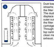
Dust loaded air streams through the filter cartridge. The dust particles displace on the outer surface of the filter cartridges. Through the open top cartridges the clean medium can
