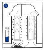
Undisturbed continuous operation is ensured by the single cleaning of filter elements. The dust falls back into the silo. At a under usage of a minimum-filter resistance, the cleaning cycle turns off automatically.
