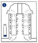
Dust loaded air streams through the filter cartridge. The dust particles displace on the outer surface of the filter cartridges. Through the open top cartridges the clean medium can exhaust.
